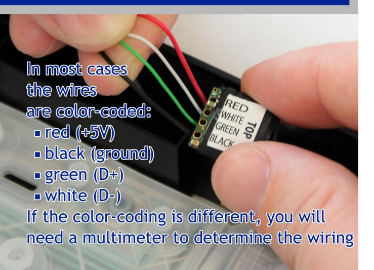
Solder the wires to the corresponding pads, melting through the isolation
