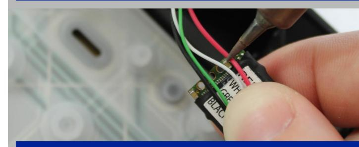
Double check the soldering, and check for short-circuits. A mistake will most likely damage the module and keyboard.
