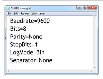
Baudrate, parity, bit count and stop bits in CONFIG.TXT must match the actual serial bus configuration
