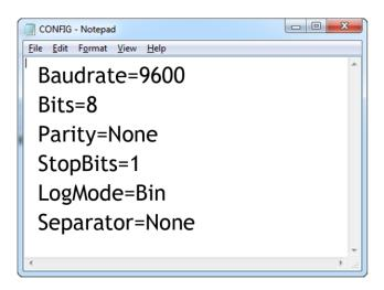
Baudrate, parity, bit count and stop bits in CONFIG.TXT must match the actual serial bus configuration
