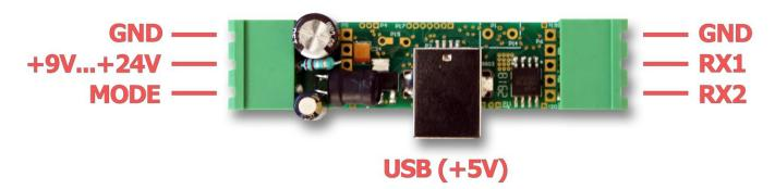
Connect up to two serial sources with RS-232 logic levels to inputs RX1, RX2
