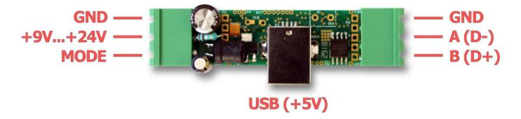
Connect the RS-485 lines to inputs respectively A (D-) and B (D+)
